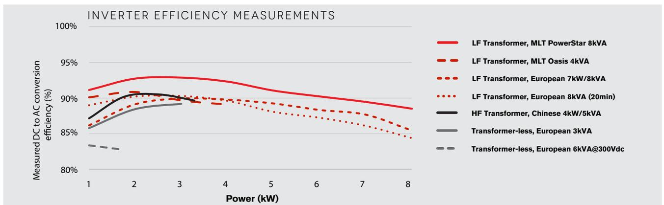
**LF Transformer** - Fewer semiconductors, transformer for safety.
